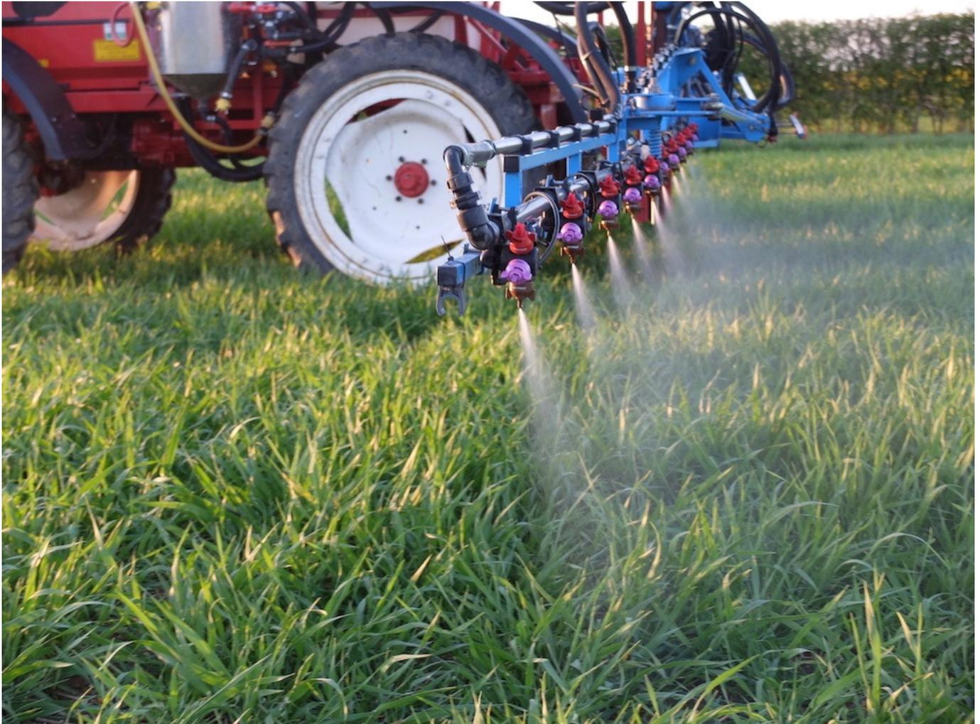
Using 75% drift reduction nozzles, rather than conventional flat fan nozzles, for flag leaf fungicide spraying can boost winter wheat yield by 0.75 t/ha, according to new Syngenta research.
